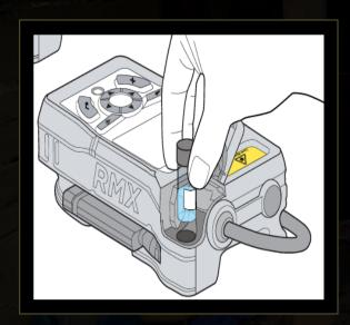
Sample vials are to be filled with disposable pipette (fancy eye dropper) and loaded into instrument as above.
