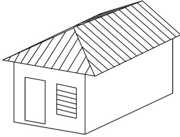
3. Replacing roof with a hip roof if re-roofing
