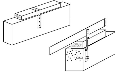
12. Strapping rafters to walls if the wall plate connection is suspect
