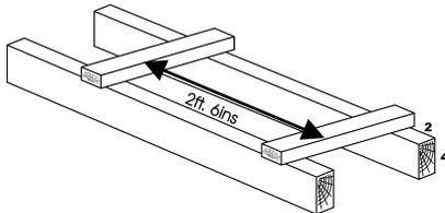
2. Raising roof pitch especially when repairing extensive damage
