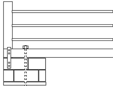
10. Strapping to foundations or building masonry footings with bolted connection
