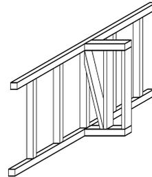
9. Adding bracing to timber walls
