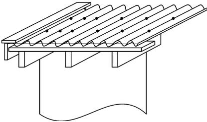
4. Boxing eaves, reducing overhangs, edge capping especially at gable ends
