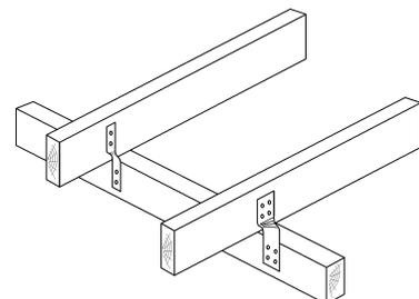
☐ Check that the purlins are less than 2 feet 6 inches (750 mm) apart, and that they are being fixed at each rafter with two nails or one screw
