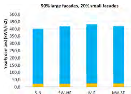
Figure 32- Yearly demand for 50% glazing on large facades and 20% glazing on small facades
