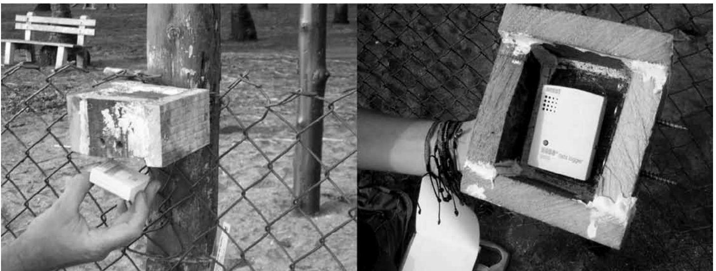
The dataloggers in semi-enclosed condition and placed 1 m above ground.
